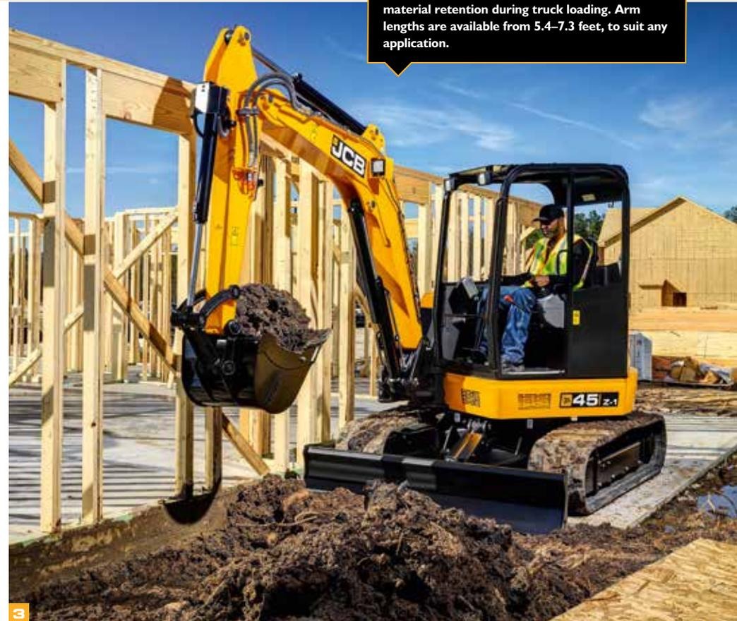
Bucket rotation is 181 degrees for maximum material retention during truck loading. Arm lengths are available from 5.4-7.3 feet, to suit any application.
